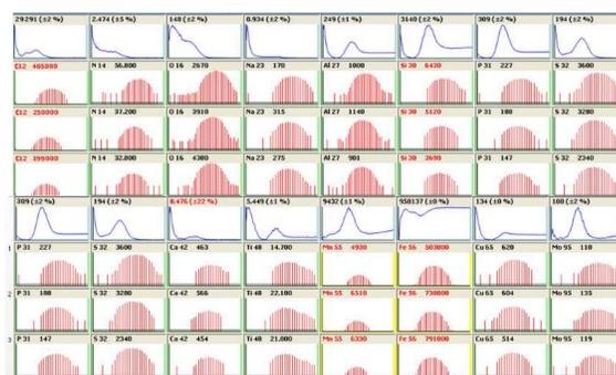
**FIGURE 3. Typical GD-OES depth profiling results of oxidized layer on low-alloy steel (Results from ISO 25138:2010 International Test Method).**
